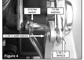
H-D, the stock inner shift arm lever may need to be gently bent in or out to properly perform this procedure. Install the  $\frac{1}{228} \times 1^{"}$  button head socket cap screw thru the rod end of the electric shift cylinder and thru the two  $\frac{1}{2"}$  flat washers and thru the Pingel shift arm lever. Put the  $\frac{1}{228}$  locknut on the backside and tighten as shown in Figure 4.
