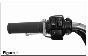
Install the dual button handlebar control bracket onto the handlebar
